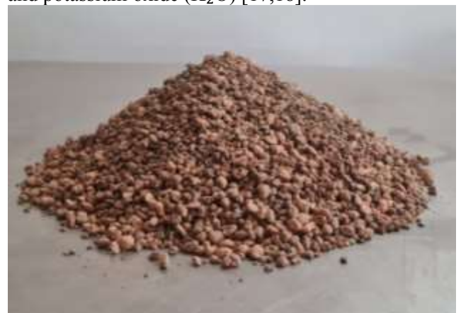
Figure 2. Physical appearance of LECA utilized as internal curing aggregate in this study.
