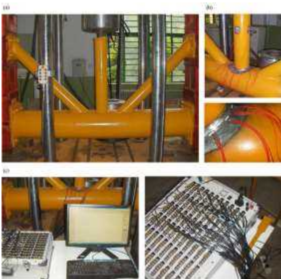
Fig. 11. Test setup: (a) View of the test rig and KT-joint specimen, (b) Strain gauges attached along the brace-to-chord intersection, (c) Connecting the strain gauges to the data logger
