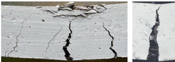
Figure 24. The BC beams crack bridging
