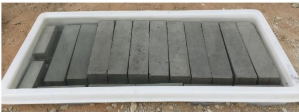
Figure 3. Drinking water curing tanks [31]
