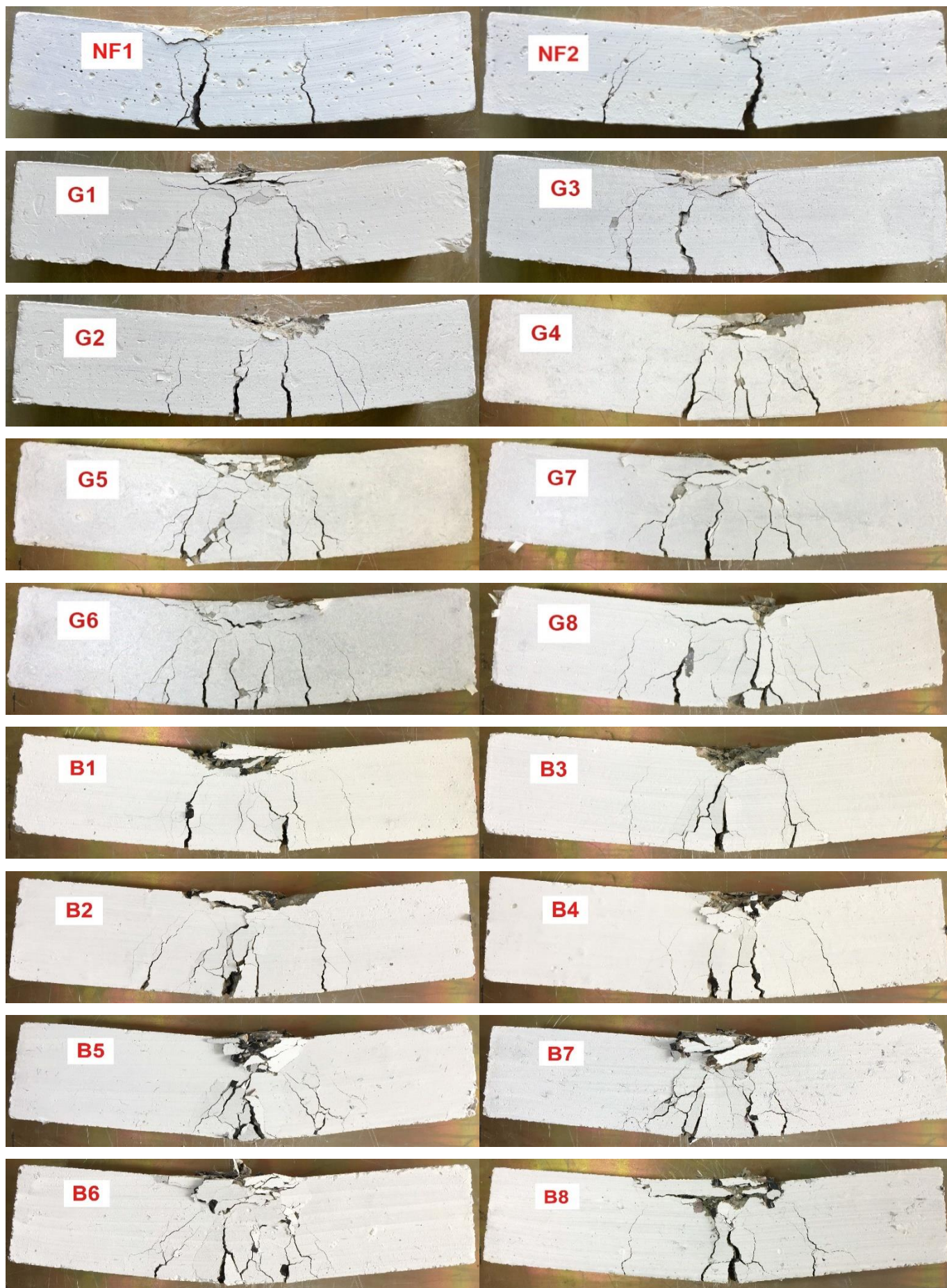
Figure 34. Cracking patterns of GC/BC beams (180 days)
