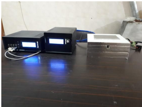
Figure 4. Device for determining the amount of reduction of nitrogen oxide adjacent to the samples in the tested designs
