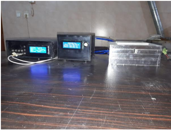
Figure 3. Device for determining the amount of reduction of nitrogen oxide adjacent to the samples in the tested designs
