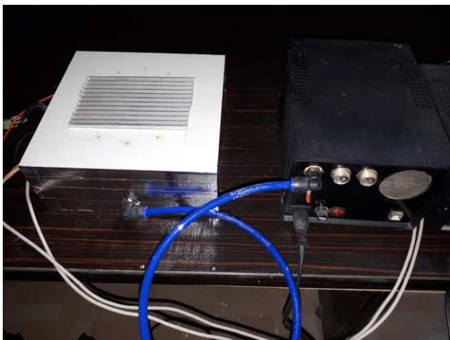
Figure 5. The input of nitrogen oxide gas from the tank to the surface of the sample in the test device to determine the reduction of nitrogen oxide adjacent to the samples in the tested designs.
