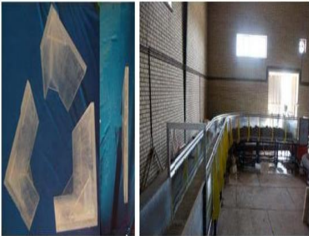
Figure 5- Schematic of the laboratory flume used and the used sluice gate samples (Divsalar and Mousavi Jahromi, 2013).
