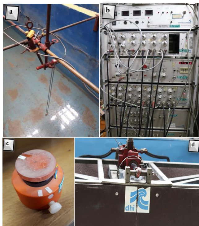
Figure 3. Measurement equipments of the present investigation; (a): Wave gauges, (b): Data logger, (c): Movement gauge, (d): Wavemaker paddel
