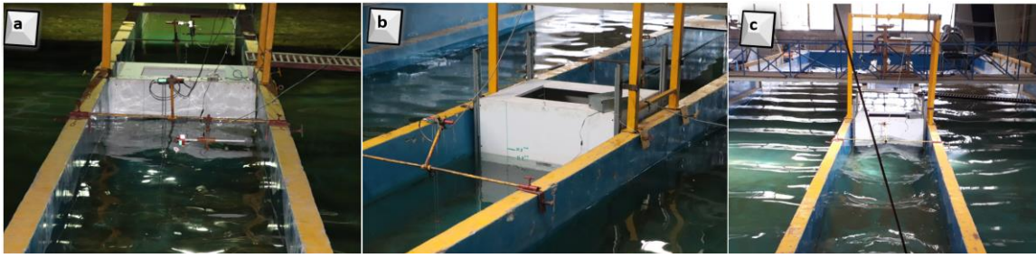
Figure 8. The installed physical model in the wave flume; (a): Anchored by cable, (b): Fixed Breakwater, (c): Anchored by chain.
