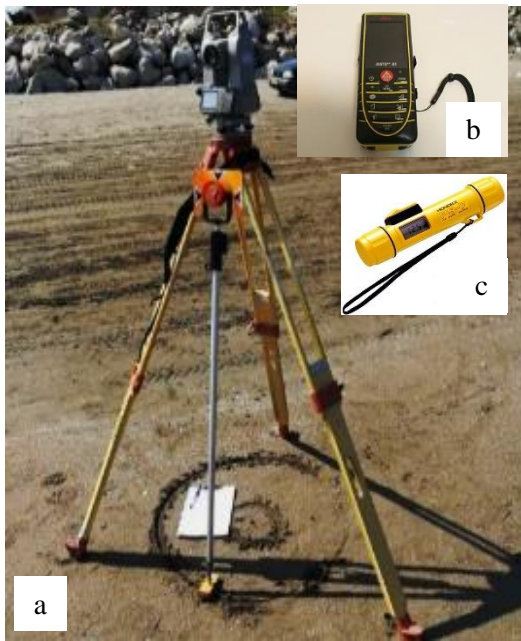
Figure 2. Theodolite mapping camera (a), GPS (b) and depth sounder (c)
