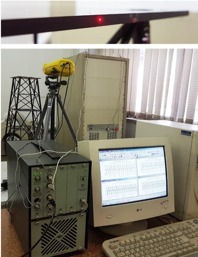
Fig. 1. Layout of the experimental test using the LDV sensing components and the scaled model.
