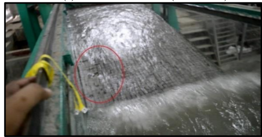
(b) Partially failed revetment (Run No: 4)
