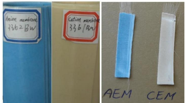
Figure 5. Heterogeneous anionic and cationic membranes of nanostructures on preservatives frames
