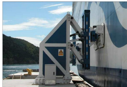
Figure1 -Moormaster unit, a commercial type [1]
