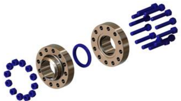
(C) Typical flanged connection (diver assisted)
