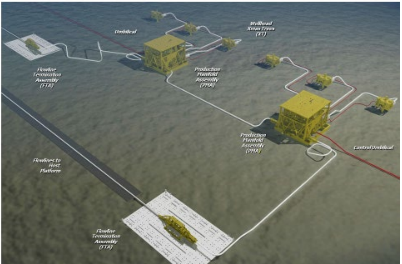
Figure 3. A cluster-type subsea architecture consisting of two manifold each connected to three X-trees.
