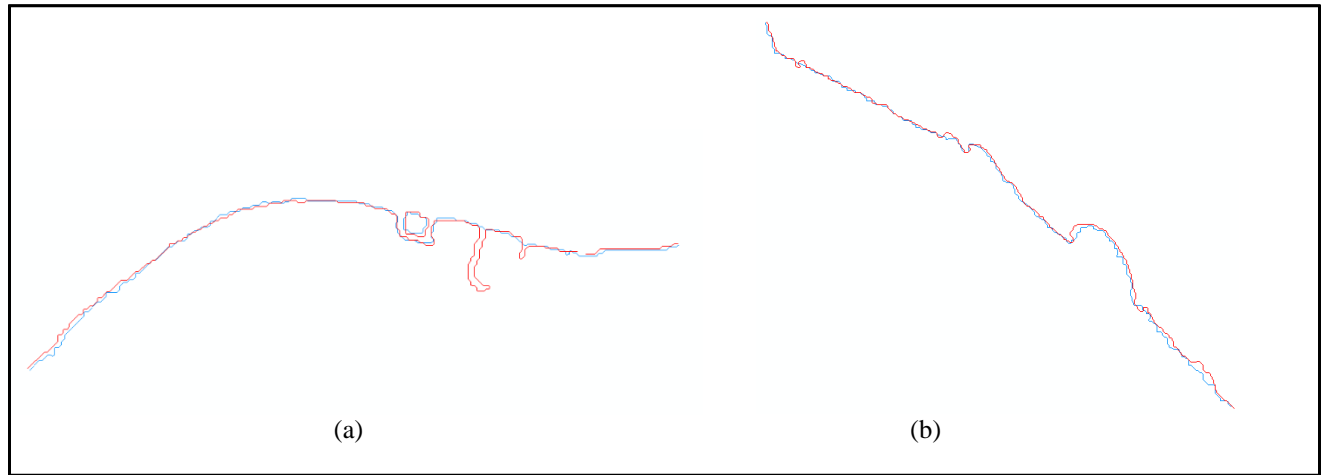
Figure 10: Coastline displacement over Qeshm (a) and Asaluyeh (b) area between 2007 (blue line) and 2016 (red line) by automated coastline extraction
