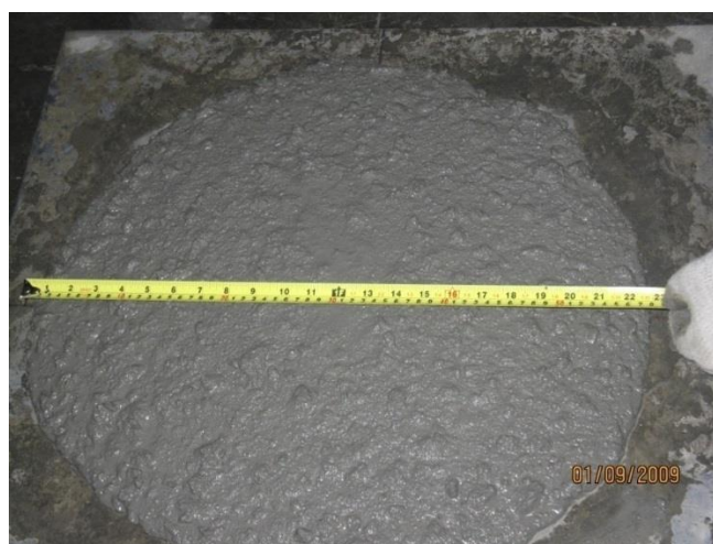
Figure 1: The flow ability of self-compacting concrete (slump=600 mm) in B1 and B2 mix design.
