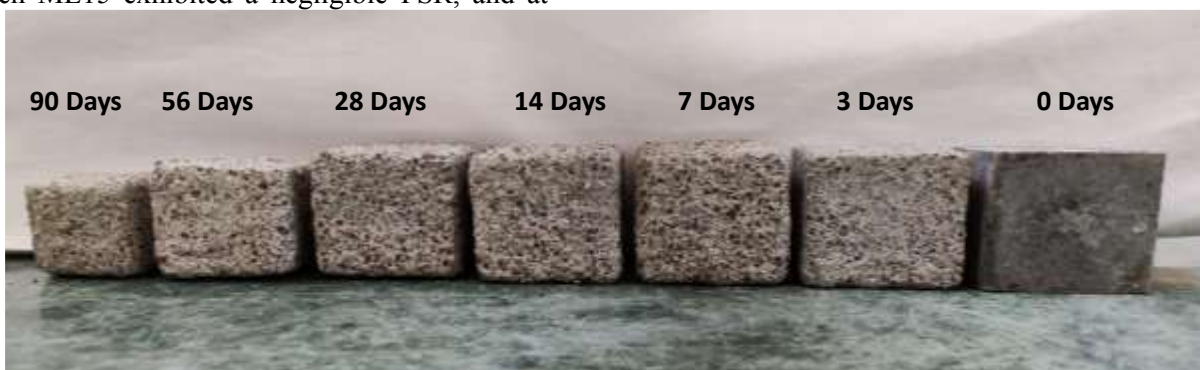
Figure 6. Surface deterioration of a cubic mortar specimen resulting from sulfuric acid exposure.
