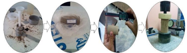
Figure (6): How to test the compressive strength in the design of different mixtures of materials
