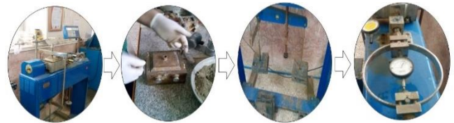
Figure (7): How to test direct shear in the design of different mixtures of materials
