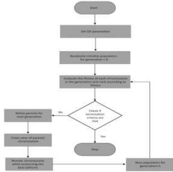
Figure 9. Flowchart of the steps of the genetic algorithm [8]
