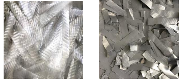
Figure 4. Strip fiber types: A) GF [31], B) BF
