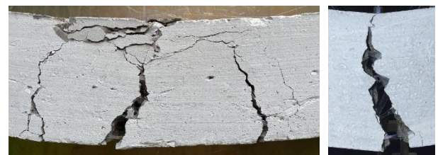
Figure 16. Crack bridging of GF in the GC beams
