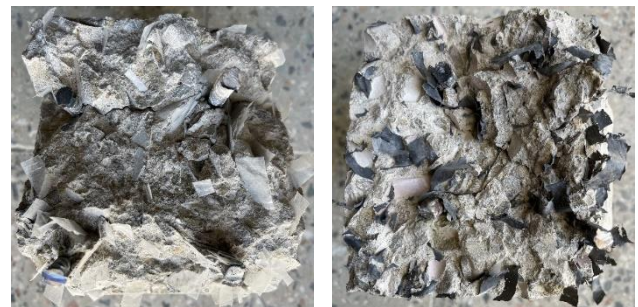
Figure 25. The cross-section of GC and BC beams
