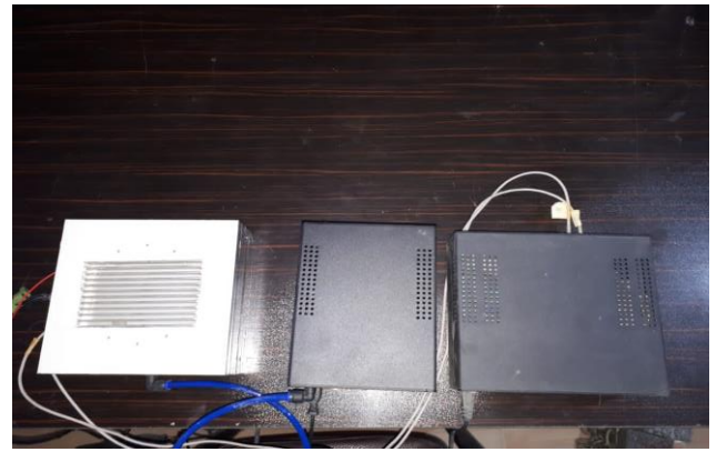
Figure 6. The output and input of nitrogen oxide gas from the tank to the surface of the sample in the test device to determine the amount of reduction of nitrogen oxide adjacent to the samples in the tested designs.
