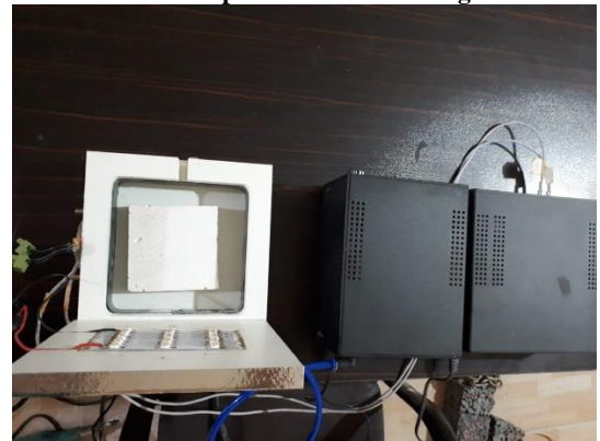
Figure 6. The output and input of nitrogen oxide gas from the tank to the surface of the sample in the test device to determine the amount of reduction of nitrogen oxide adjacent to the samples in the tested designs.
