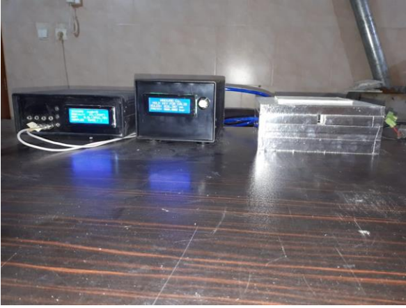
Figure 3. Device for determining the amount of reduction of nitrogen oxide adjacent to the samples in the tested designs
