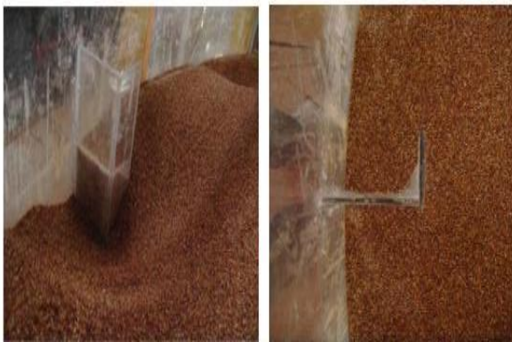
Figure 6- Example of the experiment (Sluice gate L with wing size 10.5 cm, Q=4.25 liters per second and \phi=90 degrees of bed before and after scouring (Divsalar and Mousavi Jahromi, 2013).
