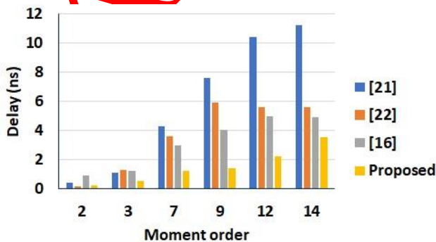
Figure 7. Comparison of delay for various moment orders in different structures.
