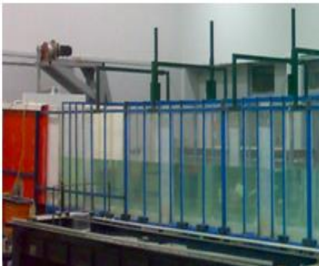
Figure 4. Total view of the wave flume in the hydraulic laboratory
