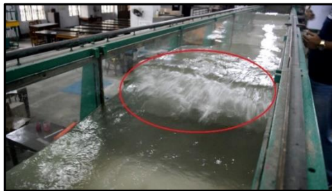
(a) Wave breaking on submerged breakwater
