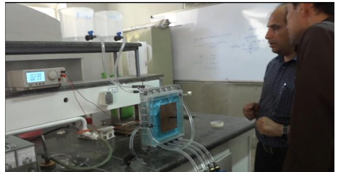
Figure 4. SGP system with nano-structured membranes used in this study
