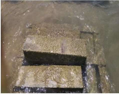
Figure 3. Beam specimens in Oman Sea environment
