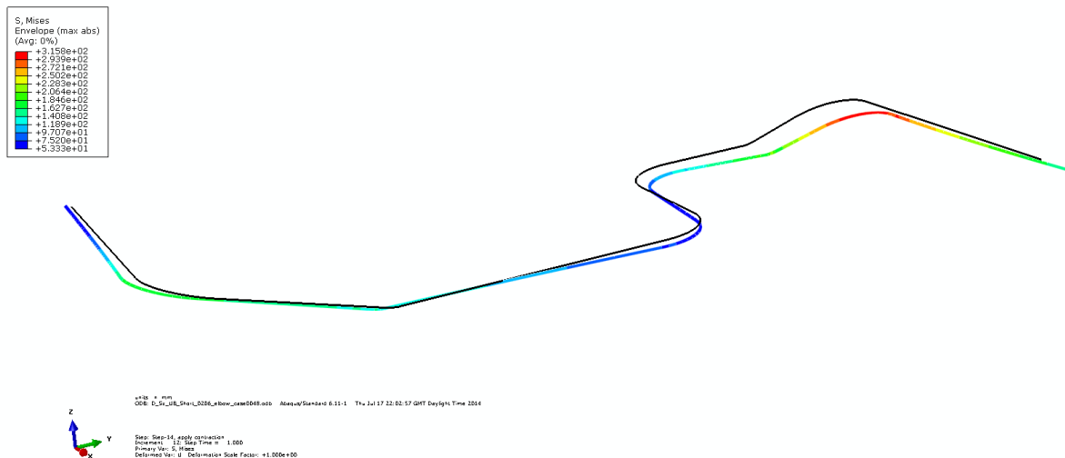
Figure11: Inner spool - Smallest Size – Envelope of Von-Mises Stress (MPa)
